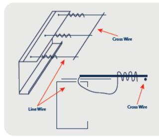
The line wire shall be attached to predrilled hole supporting metal strip member at a spacing of 150 ±5 mm. The line were shall pass through the predrilled hole on top of the projecting half of the metal strip to come around the underside of the metal strip to wrap the same line wire of the mesh on top of the metal strip.
