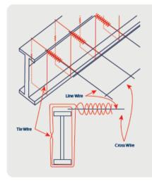
Fixing of line wires to rigid roof members by means of galvanized steel tie wires of not less than 3.15 mm diameter by wrapping the tie wire around the roof member and the wire mesh starting from the roof safety mesh side first. The middle of the tie wire must be placed at the intersection of the line wire and cross wire taking care to start at the outside of the cross wire so as to include the cross wire in the wrap process as below.
