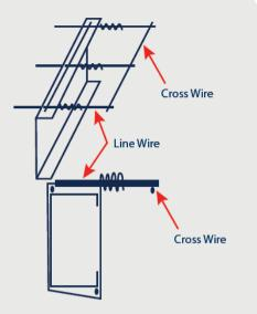
The line wire shall pass through a predilled hole at a spacing of 150  $\pm 5$  mm on top of the purlin come around the under side of the purlin to wrap the same line wire of the mesh on top of the purlin.
