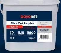
Barbed legs keep staples firmly anchored even if posts dry and split, and splayed legs and opposing slice cuts supply further reinforcement. Barbed staples are available in a range of sizes – 50mm for soft posts, 40mm for hard posts and 30mm for battens.
