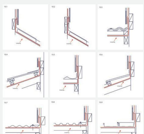
11. Aprons flashing and change in roof pitch: The underlay lap should terminate at the end of the apron flashing so as to any metal apron flashing from the supporting roof structure.
