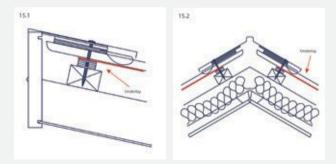
**16.** Thermal breaks: The underlay is to be installed between the roof covering and the insulating spacer to avoid thermal bridging.
