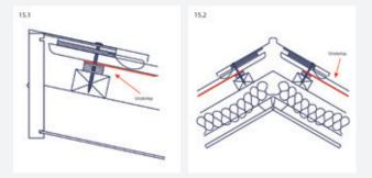
**16. Thermal breaks:** The underlay is to be installed between the roof covering and the insulating spacer to avoid thermal bridging.
