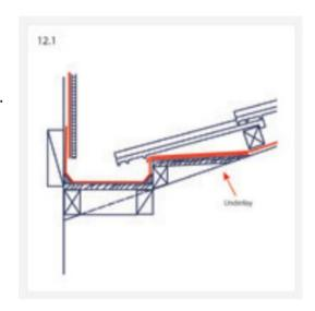
I) Parapet and enclosed balustrades: The underlay is to provide separation of the metal and timber.
