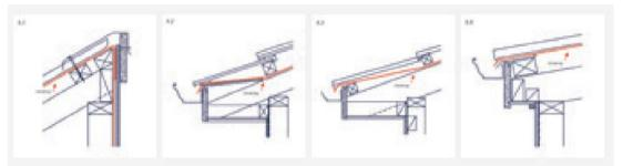
h) **Barge:** The underlay should terminate to the highest point, either the top of the barge board or meet the metal barge flashing except for horizontal profiled metal where the underlay is used to separate the metal from timber.
