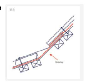
k) Abutment: The underlay is to cover the gutter lining under the roof area and overlap into the gutter by a maximum of 20mm to prevent wicking.
