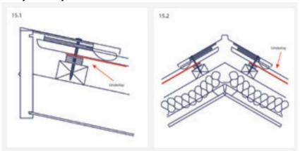
Thermal breaks: The underlay is to be installed between the roof covering and the insulating spacer to avoid thermal bridging.
