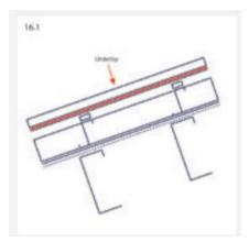
p) **Cold roofs and insulation:** In cold roof construction, the insulation is at ceiling level and there is an air gap between the insulation and the roof underlay of at least 25mm.
